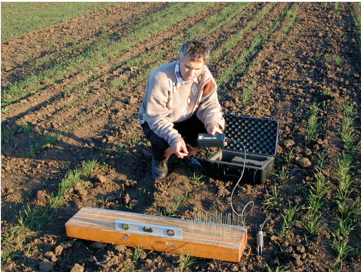
Scheme of the needle profiler for soil roughness measurements
